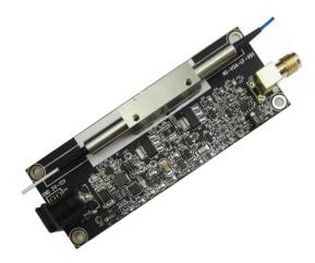
The NS VOA Driver provides driving signals for the NS series solid state VOAs. The push-pull output design ensures fast switching time for both rising and falling edges, and it is especially suitable for driving capacitive VOA loads.
